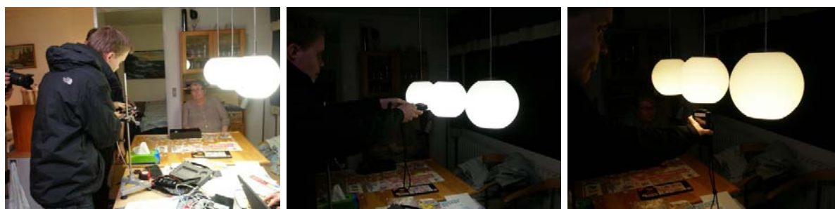
Picture 2: Spectra measurement positions. Left: Fixed position with height of 120cm, 50cm away from the lamp, towards the lamp. Middle: Approximately 2cm away from the lamp. Right: Just underneath the lamp.
