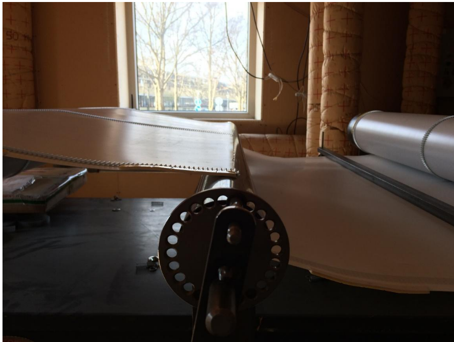
Figure 5 – Picture of preparation for the roll up of model B on the constructed roll up mounting tool. Each foil has plastic corrugated strips of 3mm in height mounted and is then rolled up on separate rolls. The foils will then be rolled together on a single roll creating a double spiral (the roll in the center of the picture).
