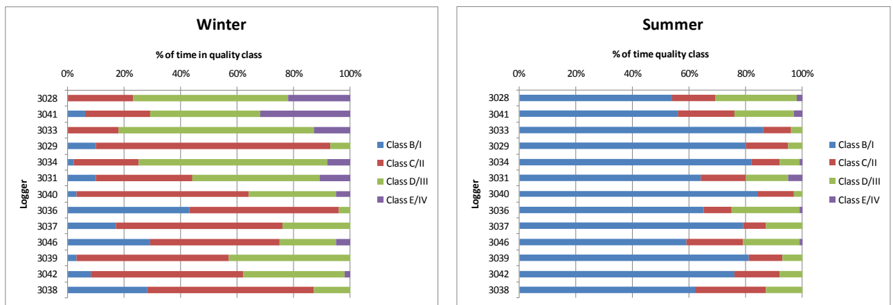
Figure 4.7. Percent of hours when the hourly mean of the measured temperature during winter (left) and summer (right) was in the ranges recommended by or DSF 3033 (2009) and CEN EN 15251 (2006) for quality classes B, C, D, E and approximately for the classes I, II, III, and IV, respectively (table 4.2 and table 4.4)
