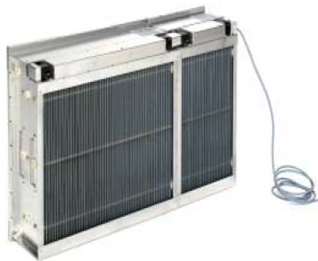
Figure 2.9: Electrostatic filter. Removes 95-99% of the ultra-fine particles. Reported power consumption 9-16 W. Source: www.automatikprodukter.se
