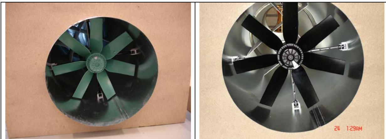
Figur 4.2 Coated ventilator i testopstilling
