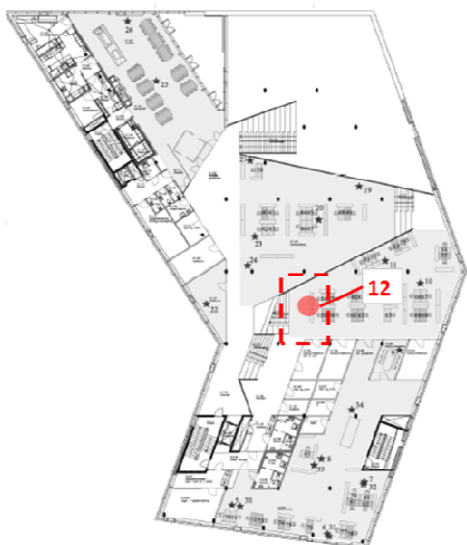
Figure 25 / Table 8 – Plateau 2 (Room 2.1.25). Area with draught risk , position of monitored point and information about the monitoring time.
