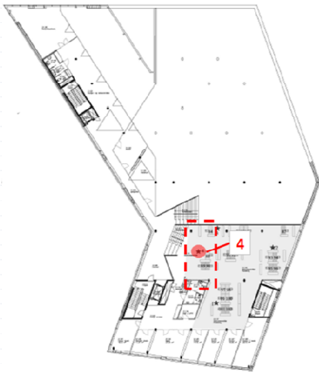
Figure 28 / Table 11 – Plateau 4 (Room 3.1.16). Area with draught risk, position of monitored point and information about the monitoring time.
