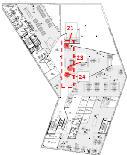
Figure 22/Table 5 – Plateau 1 (Room 2.1.23). Area with draught risk , position of monitored points and information about the monitoring time.
