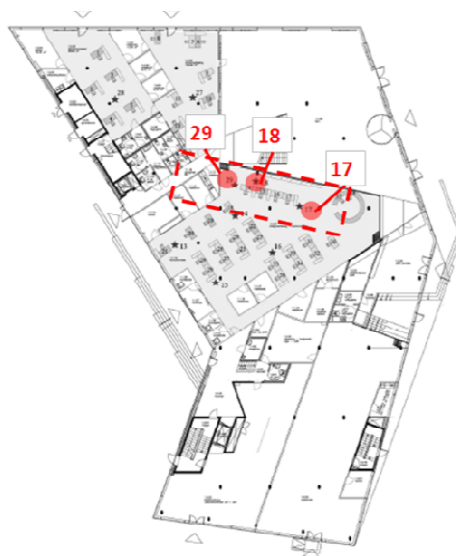
Figure 19/Table 2 – Ground Floor (Room 1.1.00). Area with draught risk , position of monitored points and information about the monitoring time.
