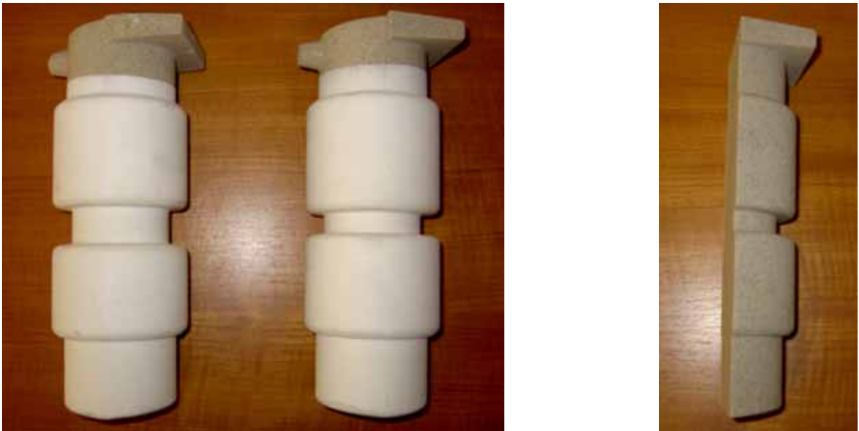
Figure 6-1 To the left: A core for the traditional layout. In the Middle: A core for the streamlined gating system. To the right: half a core used for experiments using glass plate fronted moulds.
