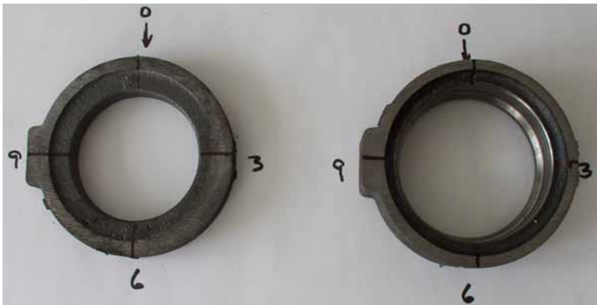
Figure 6-6 The picture shows the two centre flanges and the numbers indicates the numbering and the positions of the samples. To the left: Centre flange from the streamlined layout. To the right: Centre flange from the traditional layout.
