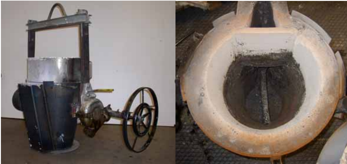
Figure 5-4 To the left: The new magnesium treatment ladle designed for 150kg of molten iron. To the right: the inside of the ladle.
