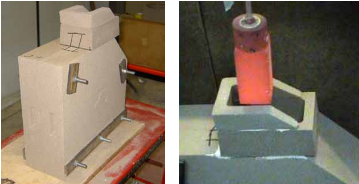
Figure 9-3 To the left: The fully assembled mould ready to be placed in the X-Ray chamber. To the right: Preheated stopper being placed in the pouring basin
