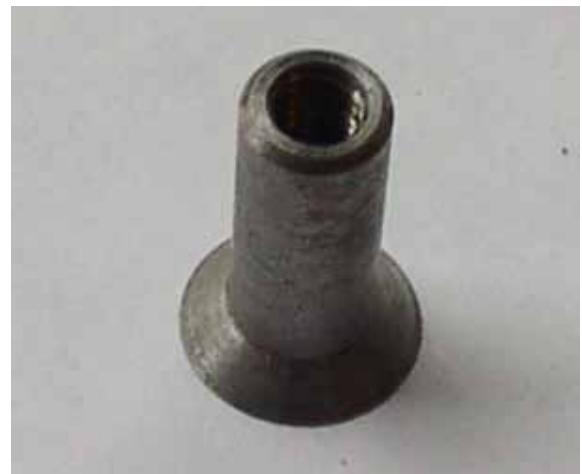
Figure 5-2 Guide pin designed for mounting the individual modules on to the base pattern plate. The length of the pin is 15mm.
