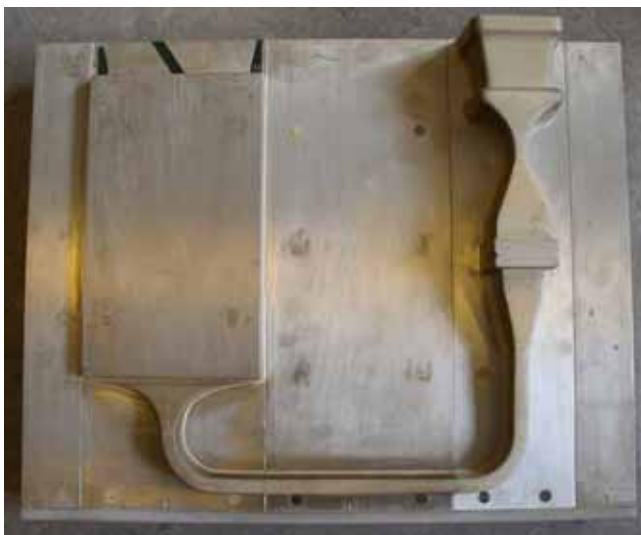
Figure 5-3 To the left: A layout consisting of three modules each going from the top to the bottom of the base plate. To the right: a close up of a module seen from the bottom. From left a part of the runner is seen. In the middle the 10mm module plate and to the right the lower part of the guide pin is seen.
