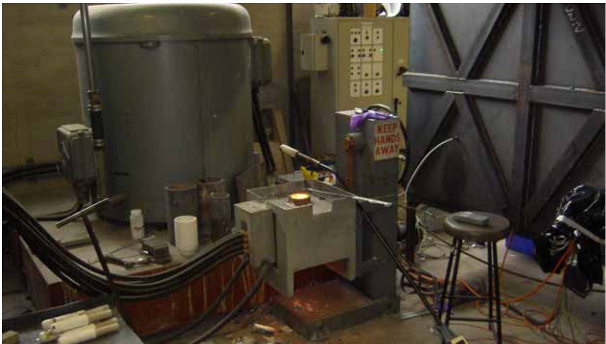
Figure 5-5 The furnace for melting
