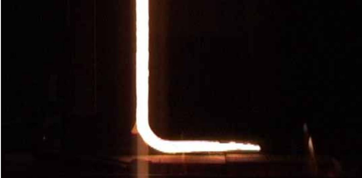
Figure 7-2 The frame shows the front of the melt in the horizontal runner. The time for the frame is 0,28s.
