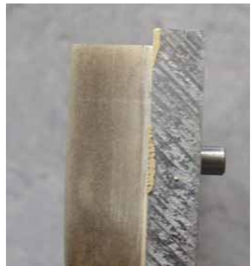
Figure 5-3 To the left: A layout consisting of three modules each going from the top to the bottom of the base plate. To the right: a close up of a module seen from the bottom. From left a part of the runner is seen. In the middle the 10mm module plate and to the right the lower part of the guide pin is seen.
