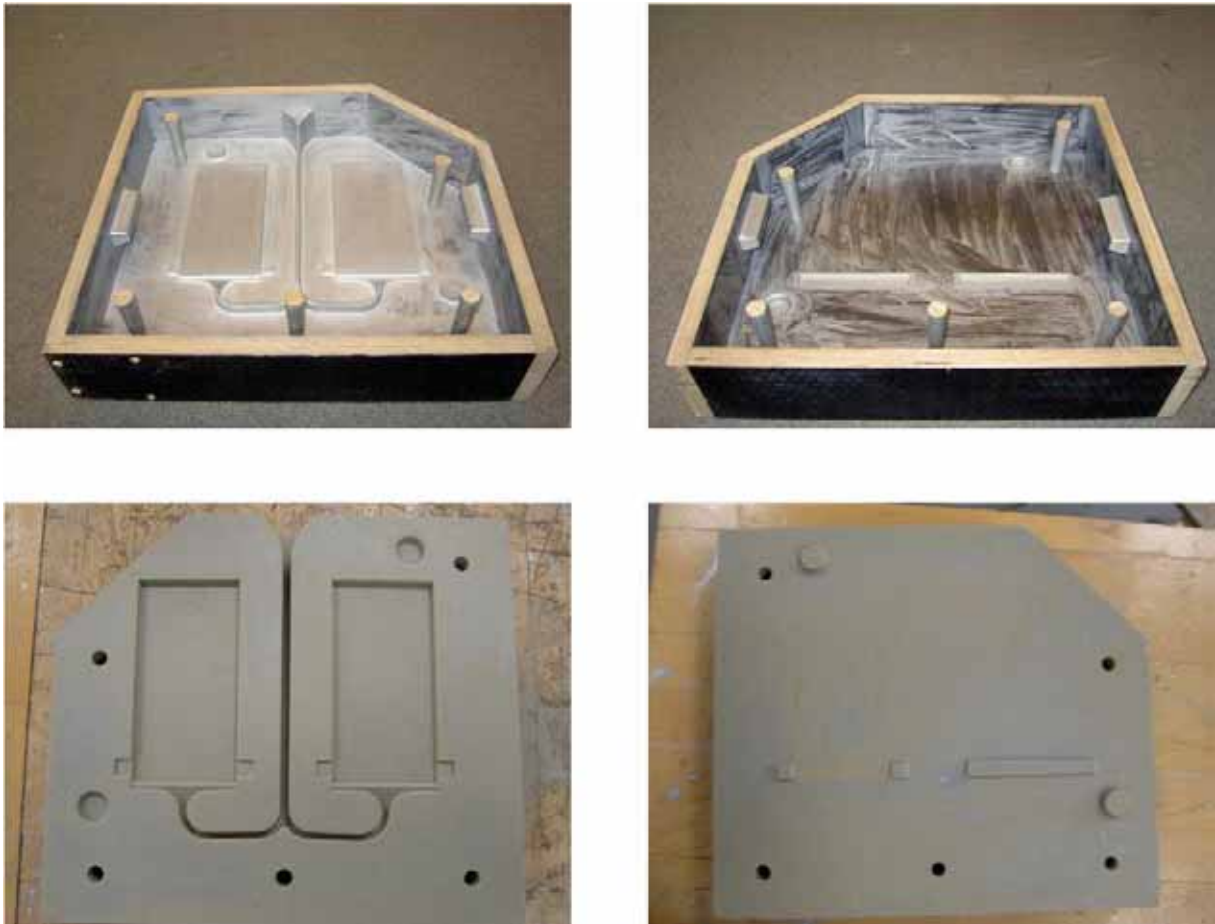
Figure 9-2 Top left: Pattern plate with the castings. Top right: Pattern plate with the ‘cores’. Bottom left: Sand mould with the castings. Bottom right: Sand mould with the core to the left removed and the core to the right intact.
