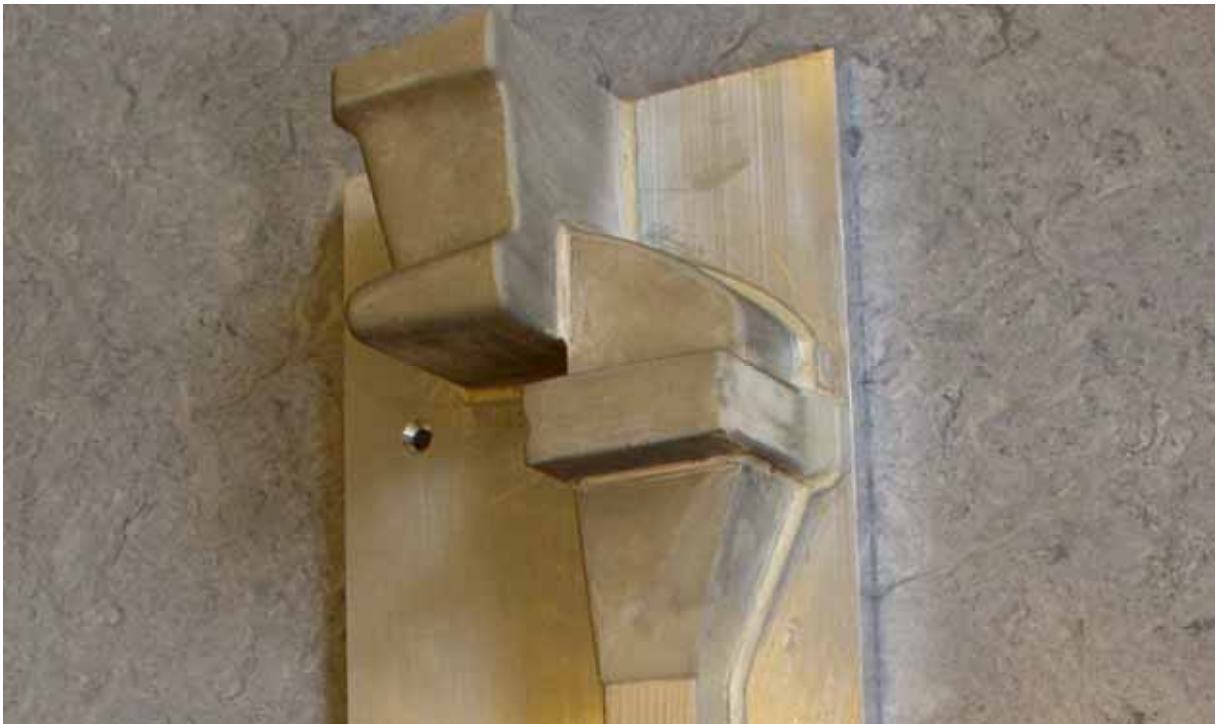
Figure 8-7 The picture show an example of how the filter prints have been slightly modified to do the glass plate experiments. In the original use of the filter print shown here the parting line would have been perpendicular to how it is used here.
