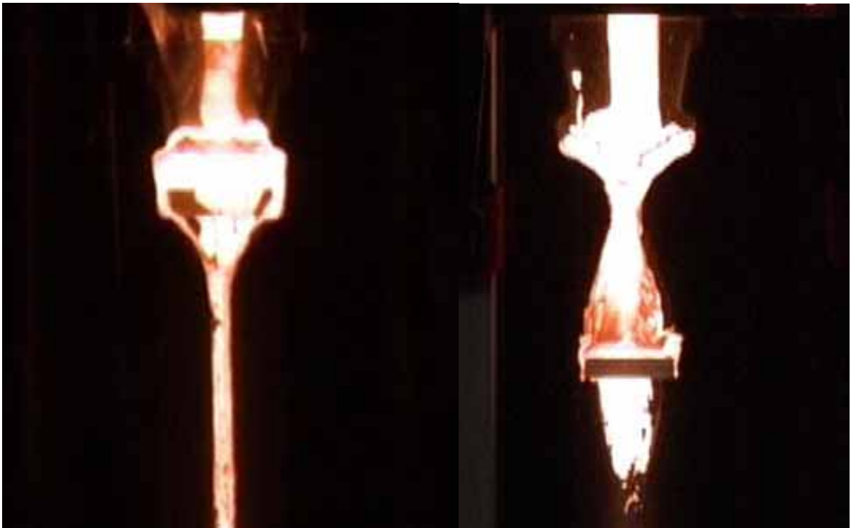
Figure 8-9 The two frames show how the melt is divided into smaller streams when using pressed filters.
