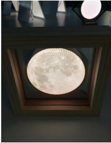
Figure 7 Round OLED panel with moon pattern from Sumitomo Chemical. Photo: DCL
