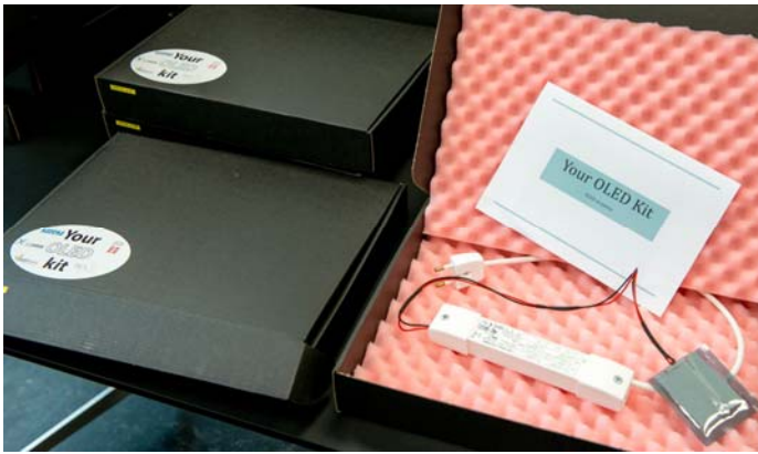
Figure 3 OLED kit consisting of an OLED panel and a driver. Photo: Carsten Dam-Hansen.
