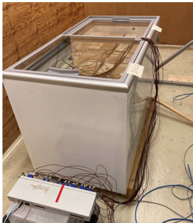
Figure 4: Prototype with the new glass lids during test at DTI.
