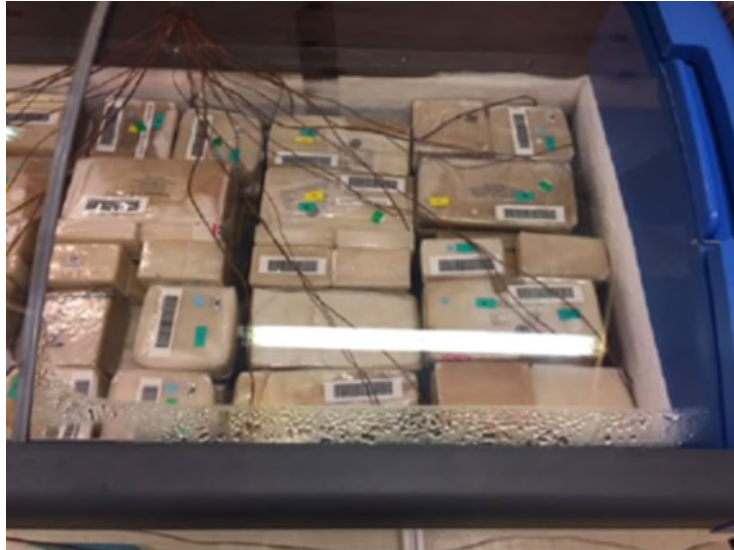
Figure 2: Test of ice cream freezer with curved glass lids in climate chamber at DTI in 2019. Due to convection under the lids, condensation takes place upon the front part of the lids since the temperature is below the dew point. In this situation the condensation test has failed, and it would be necessary to heat the front frame to increase the glass temperature.
